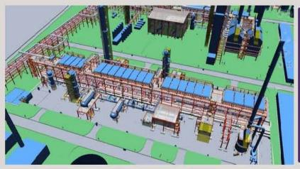
ATPL main involvement was relevant to the development of FEED and Class II Cost Estimating activities for all engineering disciplines for the Naphtha Hydrotreating Process Unit as well as 3D modelling.
